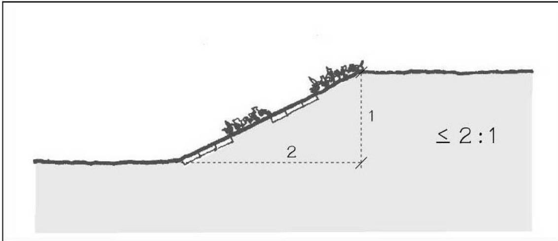
Stabilize 50 per cent or slopes greater than 2:1 with permanent slope retention devices or a suitable combination of plantings (ground cover, shrubs, etc.) and retention devices.
