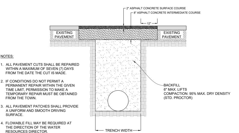
MIN: PIPE OUTSIDE DIAMETER + 8" EACH SIDE MAX: PIPE OUTSIDE DIAMETER +12" EACH SIDE
