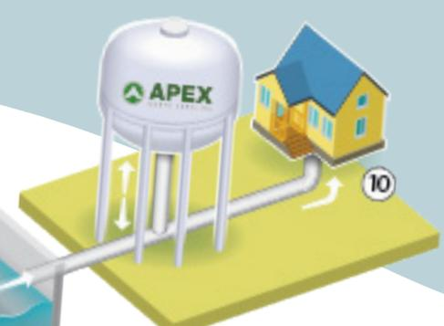
**10 Distribution System:** Water is pumped through underground water pipes in our community to water storage tanks and over 1,000 miles of smaller pipes. Elevated water tanks help maintain water pressure, ensure water is available for fire protection, and help us meet daily variations in water use.
